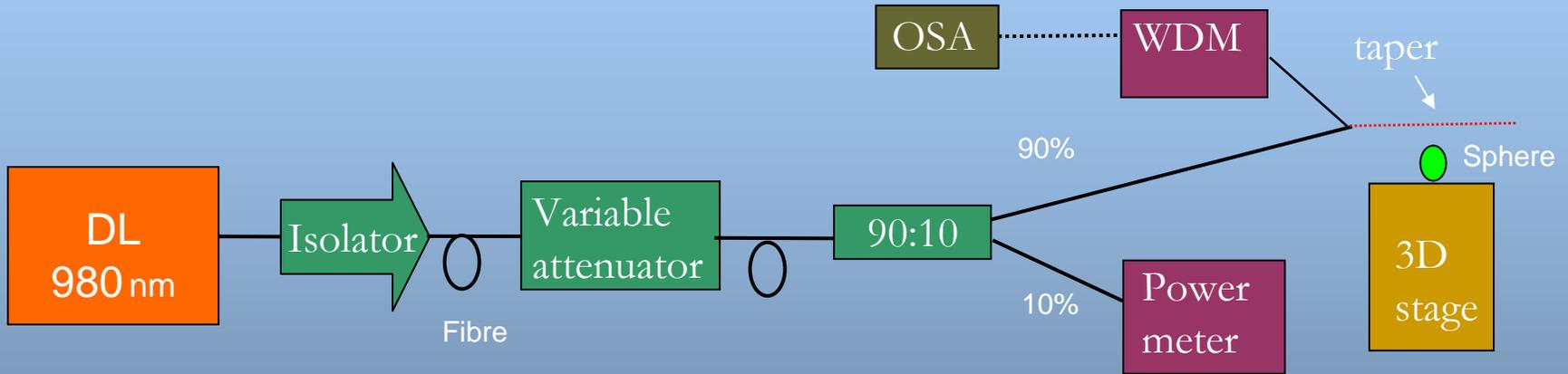
Current multimode pump source linewidth:  $\sim 17$  GHz. The same taper is used to probe for  $1.55 \mu\text{m}$  radiation by evanescent out-coupling, through a WDM and into an optical spectrum analyser.
