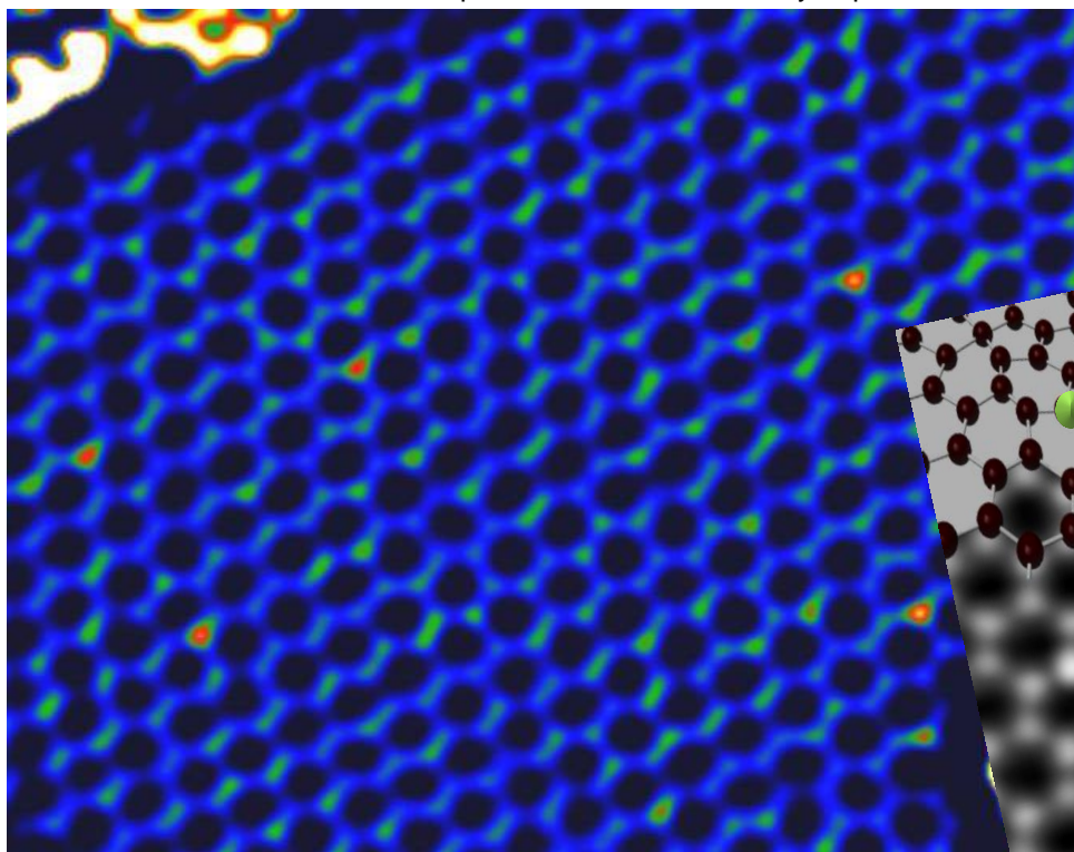
Graphene with substitutionally implanted N-atoms
