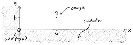
We find the potential for this system using the method of images as follows: two image charges, each with charge -q, are placed at
