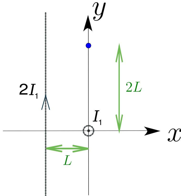
In the first wire (running along the  $z$  axis), the direction of current is perpendicular to the page, pointing outward from the plane of the paper (toward the reader). Why outward toward the reader, and not inward into the page? Because the  $z$  axis points outward from the plane of the paper, and the question specifies that the current flows from  $z = -\infty$  to  $z = +\infty$  through the origin.
